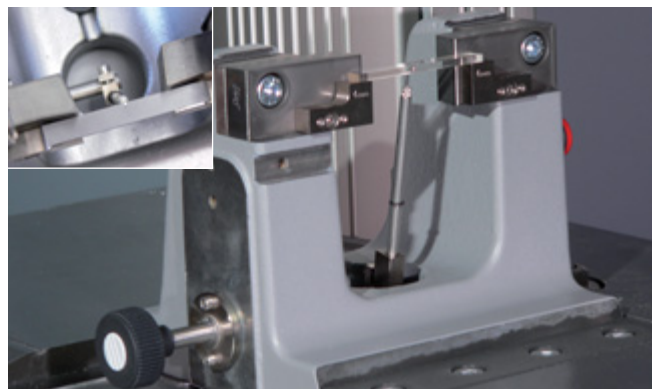
Fig. 3: Notch alignment unit on Charpy fixture
