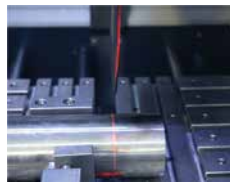
Laser alignment unit (for MA & AA models)(To be ordered simultane- ously together with the machine order)
