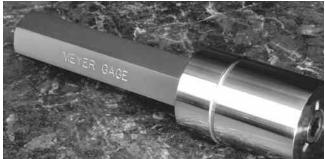
When you need to check parts quickly, Progressive plug gages are the best choice. Both the GO and NOGO diameters are stepped on a single gage member. All members are securely attached to either a trilock or taperlock handle. All handles are marked with sizes and direction of tolerance.
